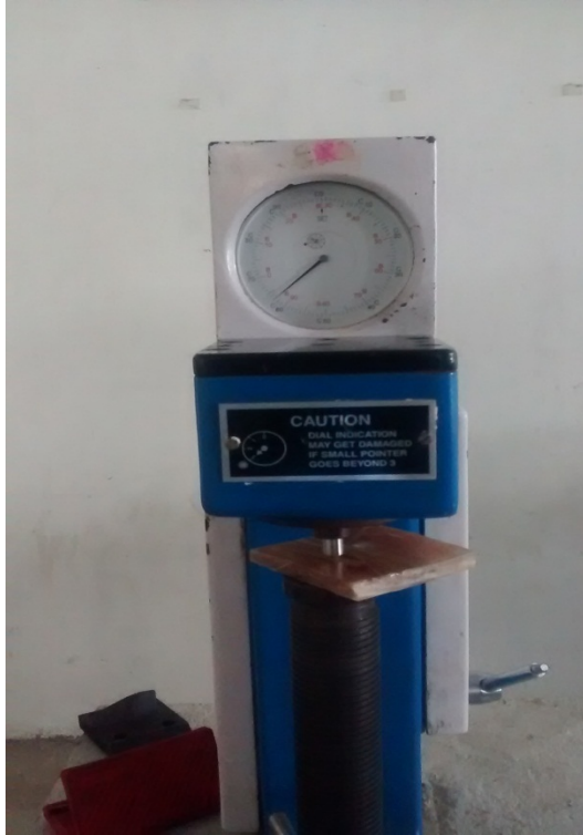
Fig. 7: The photographic view of Rockwell hardness testing machine used for this study
