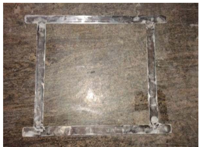
Fig. 3: Mould fabrication with a mallet sheet of 50*50 cm size
