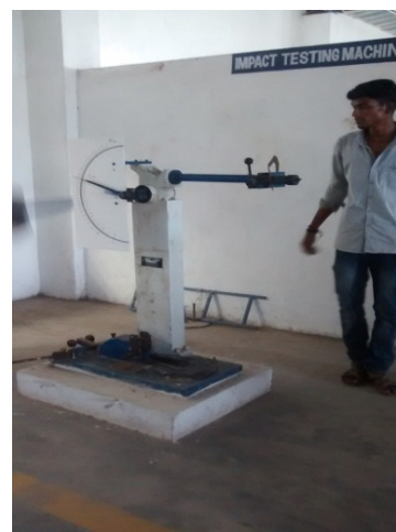
Fig. 6: The photographic view of impact testing machine used for this study
